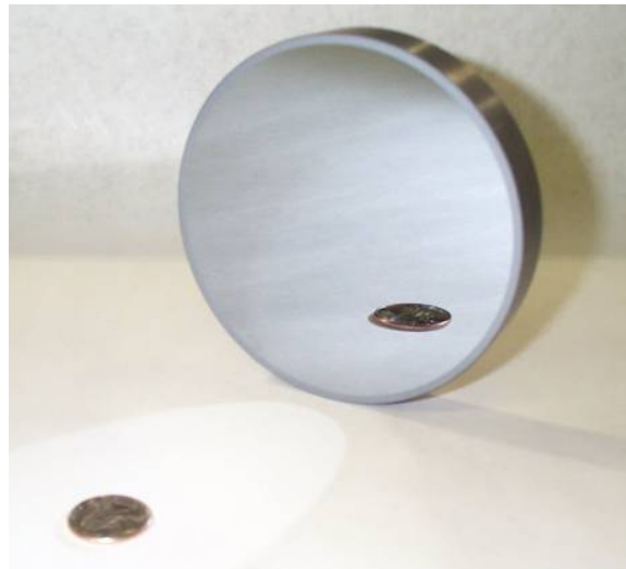
Figure 3: Glass Frit Bonded Spherical Lightweight Silicon Mirror
