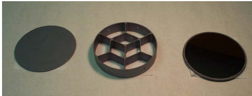
Figure 2: Elements of lightweight silicon mirror illustrate simplicity of design
