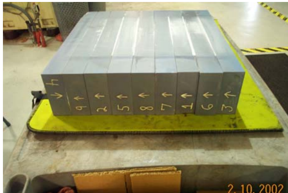
Figure 8: Silicon Frit Bonded Sub-assembly before Sawing
