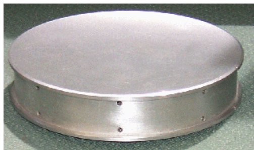
Figure 6: McCarter Prototype Frit Bonded Mirror
