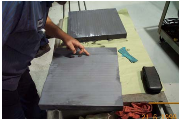
Figure 9: Silicon Frit Bonded Sub-assembly after Sawing
