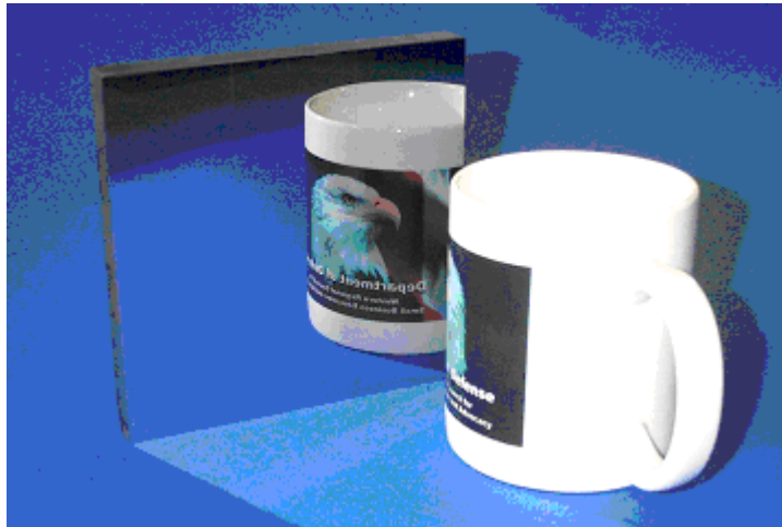
Figure 2: Flat Silicon Mirror Composed of Three Planks
