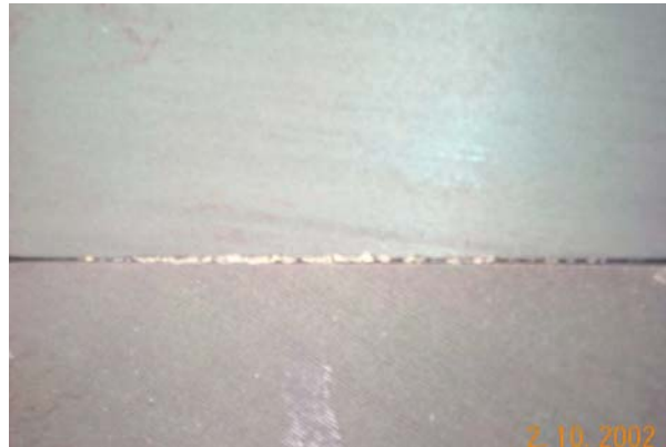
Figure 13: Frit bonded Joint
