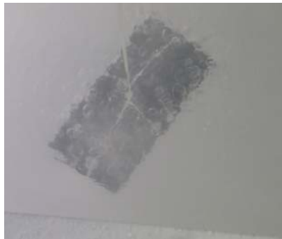
Figure 4: Submerged Frit Bonded Silicon Planks
