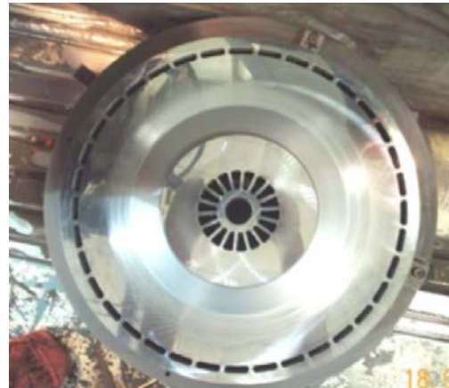
Figure 4. Slotting and boring across frit-bonded 711mm structure.
